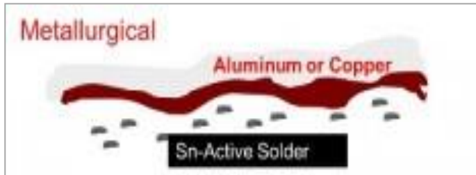
Figure 1 - Illustration of Metallurgical Bond Formation
