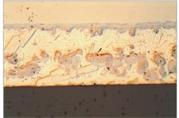
Figure 2 – S-Bond - Aluminum Bond Interface
