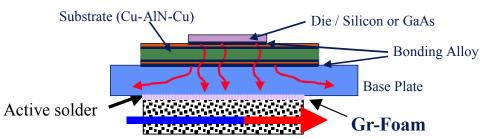
An example of thermal foams bonded to electronic packages is shown to the left. NOTE: S-Bond can be used to bond all the interfaces, including: Si / AlN or Al<sub>2</sub>O<sub>3</sub> / Metal Base / Gr-Foam.
